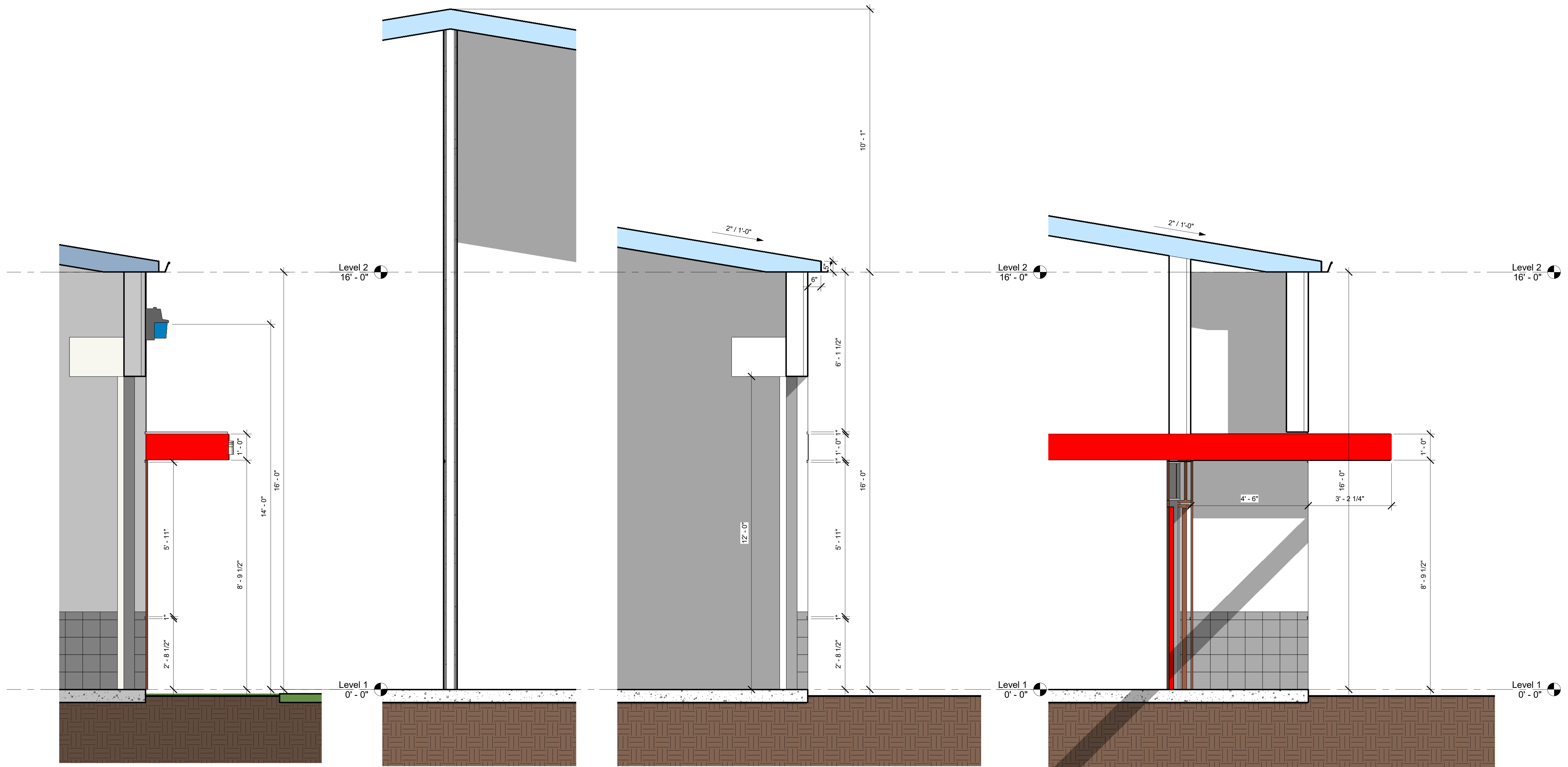
① Wall Section at Entry Door 1/2" = 1'-0"
